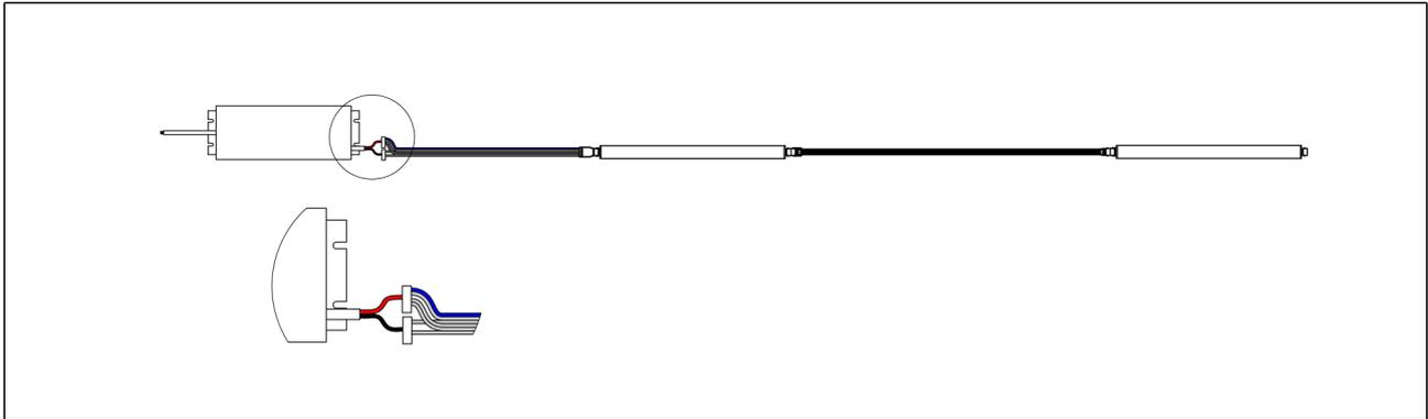
**+36 VDC power supply connect to wire 1 (marked blue), wire 2, wire 4, wire 5 of the leader cable**
