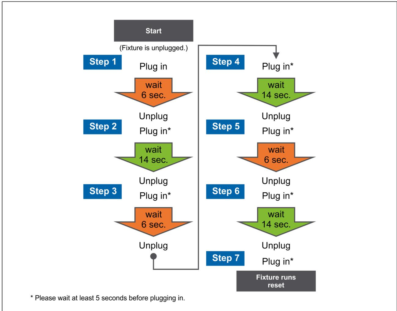
In case that a BION TECHNOLOGIES IOTcontrol device appears unresponsive, please check first that the fixture is correctly wired and powered. Please unplug the device for 10 seconds from the mains, then power up again the unit for a restart of the fixture.
